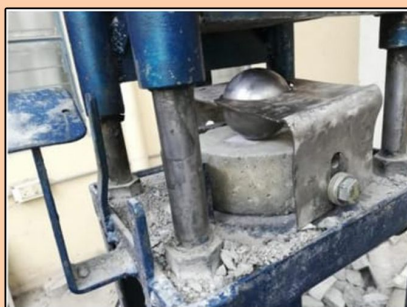
Steel ball at centre of specimen
